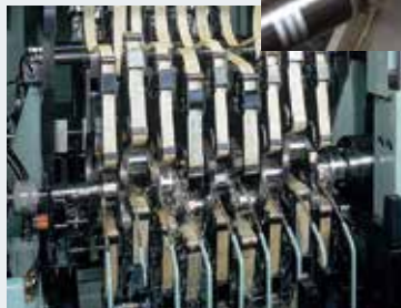
Power Finisher Crankshaft and camshaft lapping.
